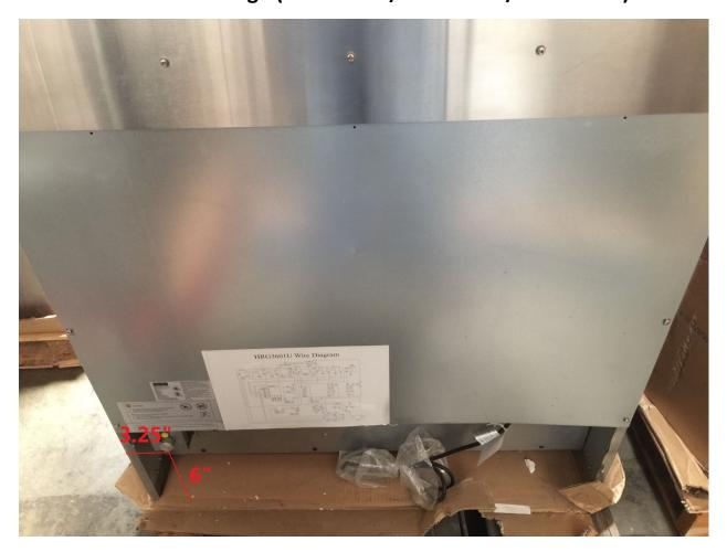
Distance from inlet gas pipe to right side of the range is 3.25".
