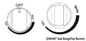
To light the top burners, push and turn the appropriate control knob counter clockwise to the "HI" position. You will hear a clicking noise – the sound of the electric spark igniting the burner. Once burner ignition has been achieved, then turn the burner control knob to adjust the desired heat setting.
