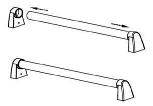
3.3 Lay the door handle against to the oven door and fit it on the connection part, and use the wrench to get the door handle holder tight;
