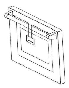
3.4 Use the wrench to tighten the door handle holders.
