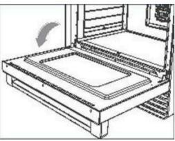
4. Fully close the levers on the left and right hinges, as shown, then close the door.
