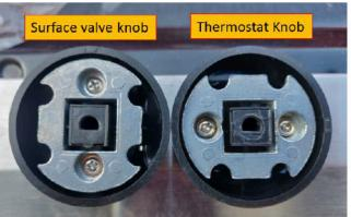
(Incorrect knob caused broken thermostat shaft)
