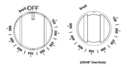
To light the oven burner, push and turn the appropriate control knob counter clockwise to the  $(150\sim500)$  position. You will hear a clicking noise – the sound of the electric spark igniting the burner. Once burner ignition has been achieved, then turn the burner control knob to adjust the desired heat setting.
