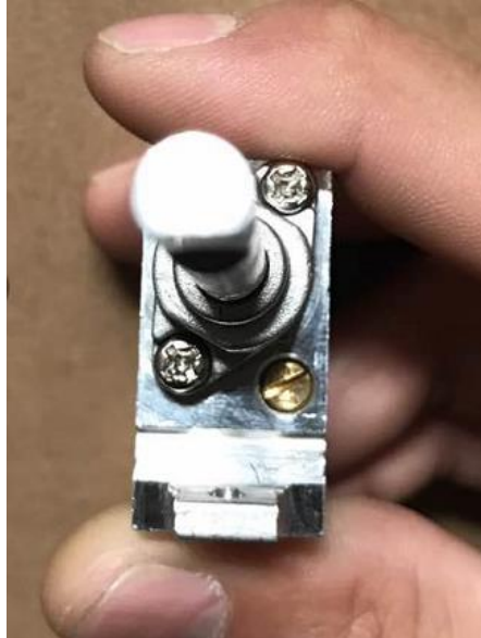
(Gas Valve and they yellow brass bypass orifices)
