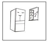
The refrigerator is placed in a well-ventilated indoor place; the ground shall be flat, and sturdy (rotate left or right to adjust the wheel for leveling if unstable).
