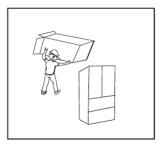
Before use, remove all packing materials, including bottom cushions, foam pads and tapes inside of the refrigerator; tear off the protective film on the doors and the refrigerator body.
