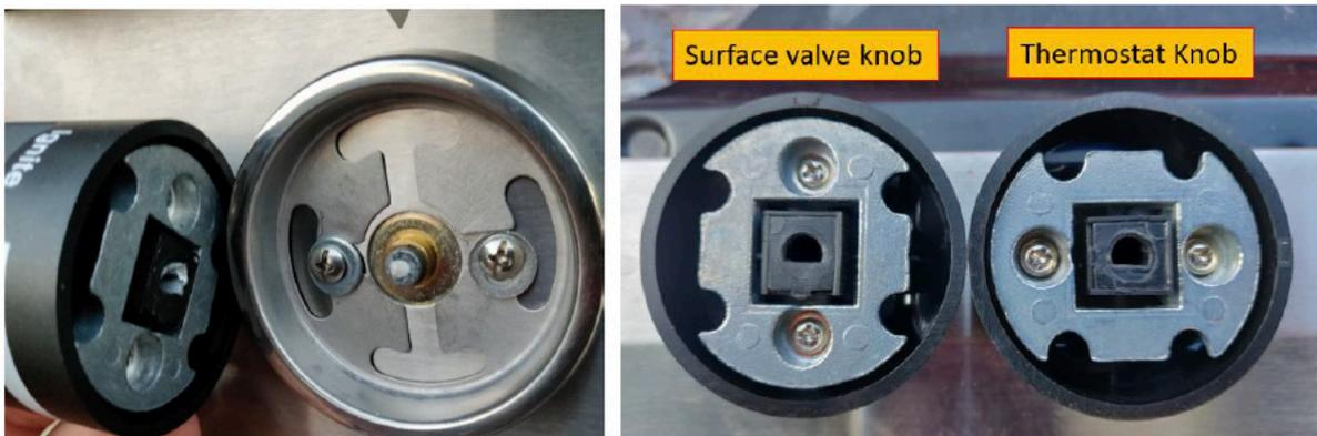
(Incorrect knob caused broken thermostat shaft)
