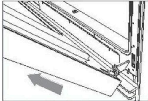
4. Disengage the hinges and remove the door, gently close it about halfway, place on a protected surface.
