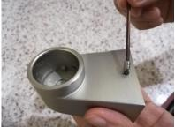
4. Mount one end of the door handle into the holder, making sure the notches insert correctly;
